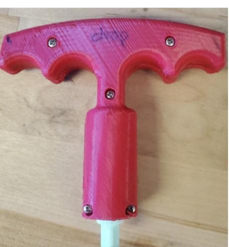
In conclusion, the most important problems this torque wrench could rectify are issues that current industry wrenches cause. Torque wrenches currently on the market rarely ever hit their manufacturing set torque limit even within a plus or minus 10% range. The main issues a disposable torque wrench will solve are lowering cost, increasing the accuracy of pre-set torque values and ease manufacturing processes for PMI while also improving
