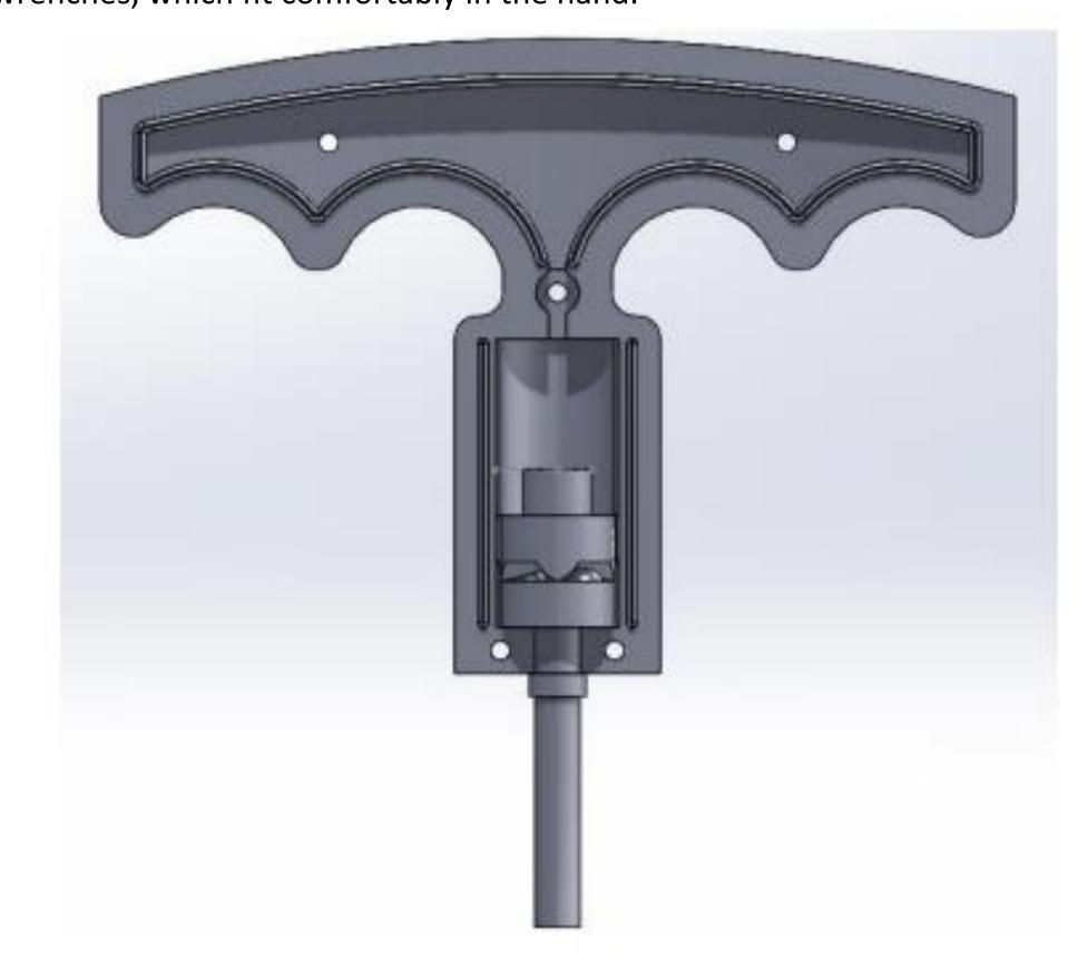
The two internal pieces were designed to interface with one another and at their peaks, the proper torque value will be outputted. The spring rests on top of the resistance plate and is further compressed when a torsional force is applied to the handle. Redesigns of the internal components included reducing diameters for better clearance, increasing thickness to increase compression, and changing the shaft end to accommodate for the testing methods required.
